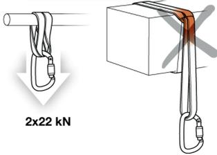
**Tested tensile strength**
