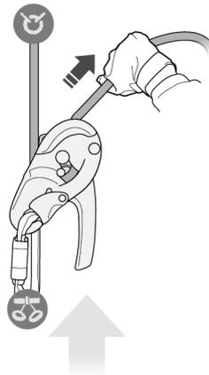
10e. Always hold the brake-side rope when the climber is moving.
